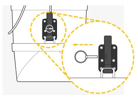
**1.2.4** Rope is removed from the bag strap and uncoiled such that the operator may stand at a safe distance before pulling to the cord to release the bag.
