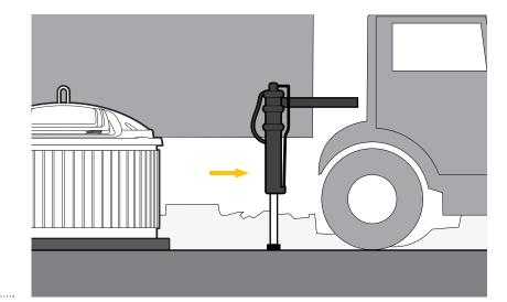
**2.1.3** Extend the crane and attach the chain hook to the loop on the top off the bin
