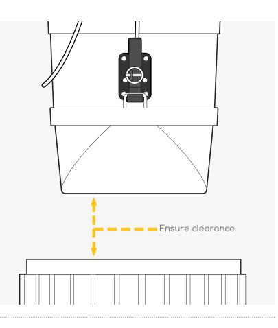
**1.2.2** The operator ensures that the bag does not contact any obstacles while bag is moved to the truck hopper in preparation of being emptied.
