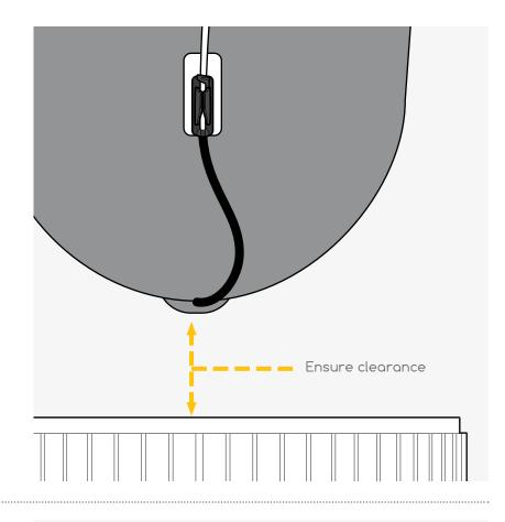
**2.2.2** The operator ensures that the bag does not contact any obstacles while bag is moved to the truck hopper in preparation of being emptied.
