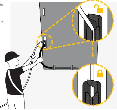
**2.2.8** The release rope is then coiled and affixed to the strap or placed into the storage pocket.
