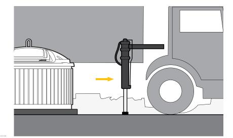
**1.1.3** Extend the crane and attach the chain hook to the loop on the top off the bin
