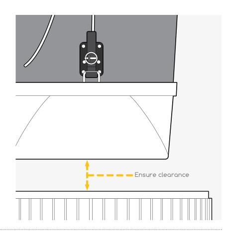
**1.2.2** The operator ensures that the bag does not contact any obstacles while bag is moved to the truck hopper in preparation of being emptied.
